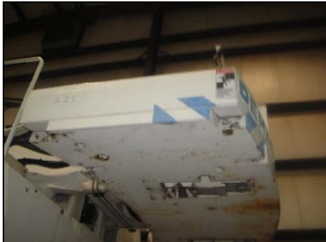
The base counterweight of a mobile crane without the removable counterweights that should be mounted to develop the full crane lifting capacity without tip over.
