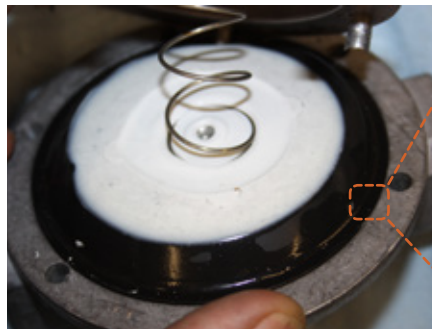
FIGURE 9 Regulator from Test 4-A. No degradation of POM diaphragm plate. Melted but not discolored or embrittled.
