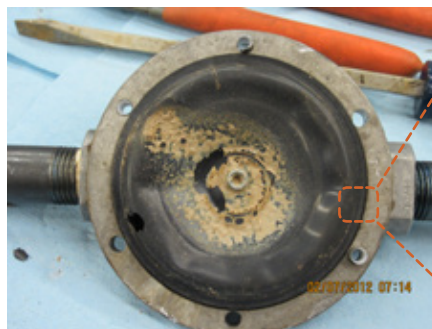
FIGURE 10 Regulator from Test 8-A. Extensively degraded POM diaphragm plate with significant mass loss. Substantial hardening and embrittlement of NBR diaphragm plate. Note the fracture on the lower left side.
