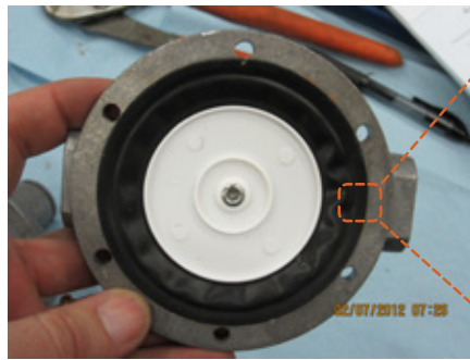
FIGURE 8 POM diaphragm plate from an untested regulator.
