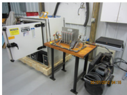
FIGURE 6 Oven exposure test set-up.
