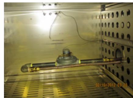
FIGURE 7 Oven exposure test set-up.
