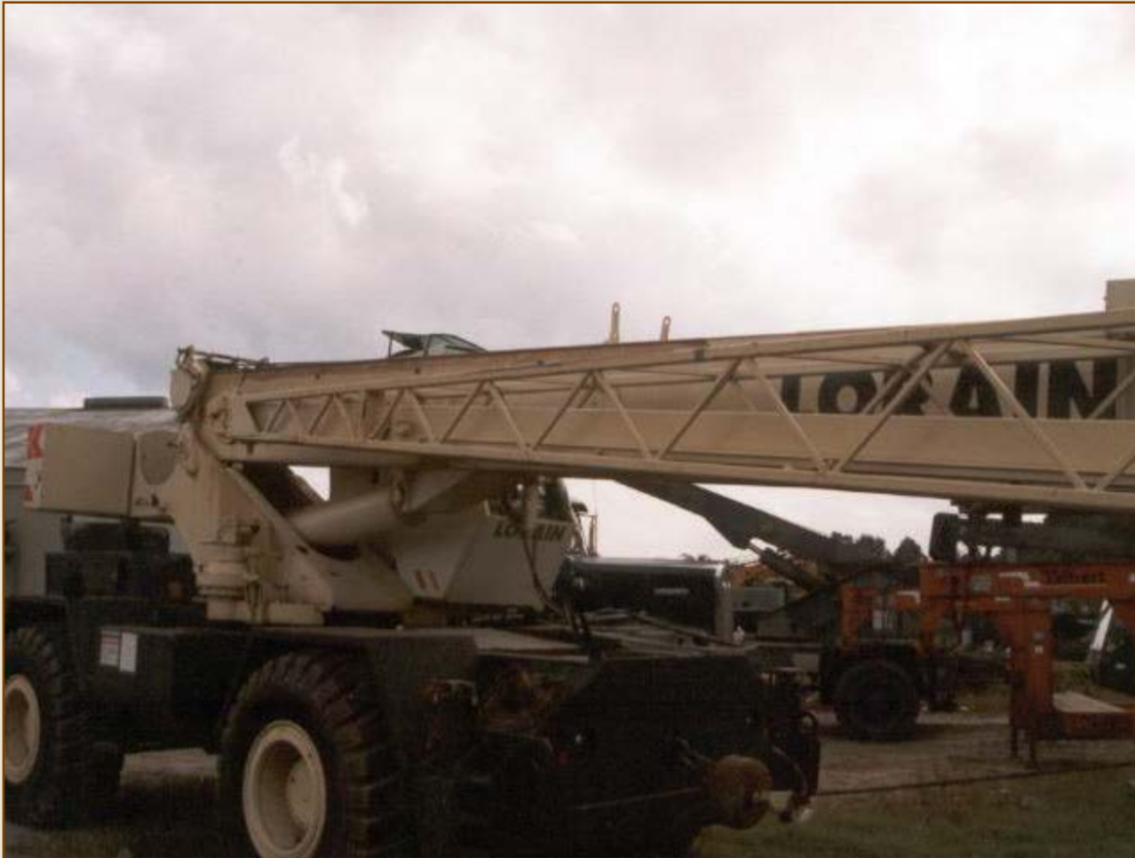
A rough terrain crane that swung unexpectedly while operating on a slope, damaging the crane boom.
