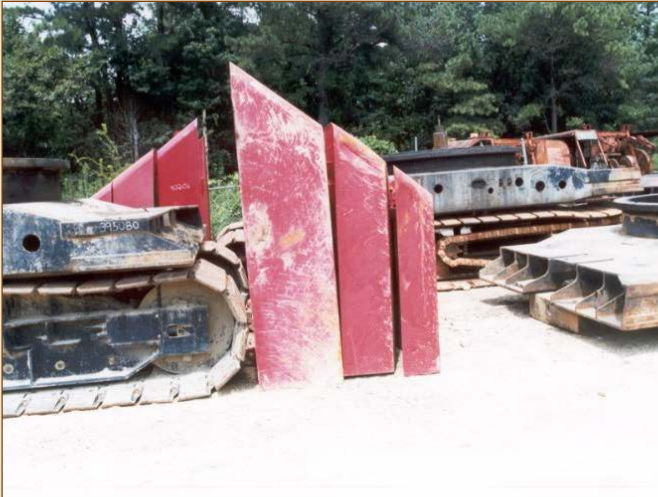
Removable crane superstructure counterweights. Different numbers of these counterweights will be installed depending on the crane loading.
