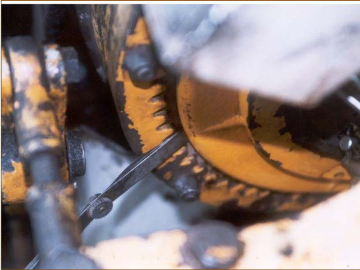
Boom hoist drive clutch measurement on the same friction crane.
