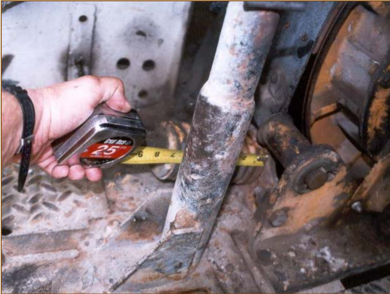
Brake adjustment measurement on the friction crane in the previous photograph.
