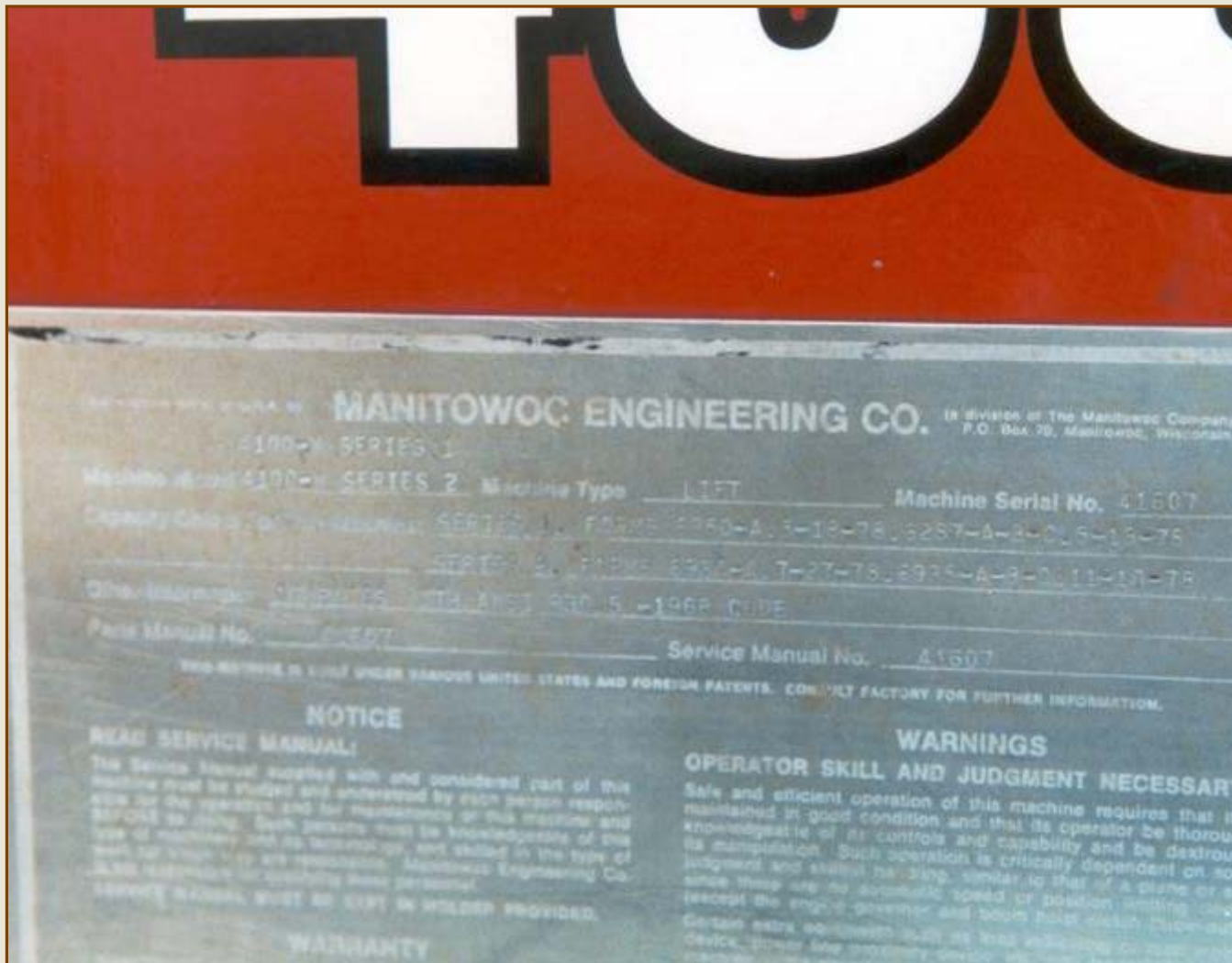
A typical crane label identifying the manufacturer, model number, and serial number.
