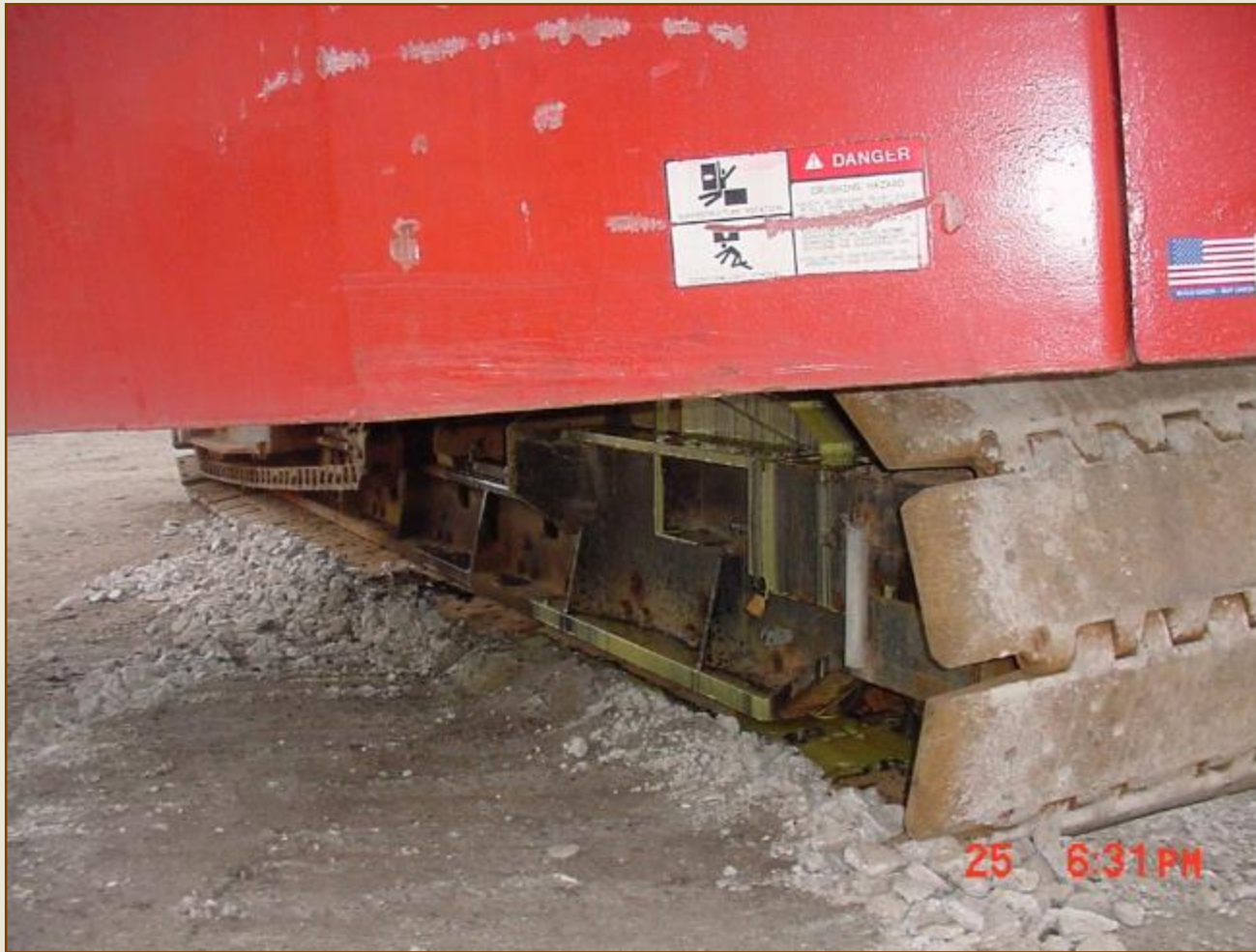
Impressions showing good soil support of a crawler crane after an overload incident
