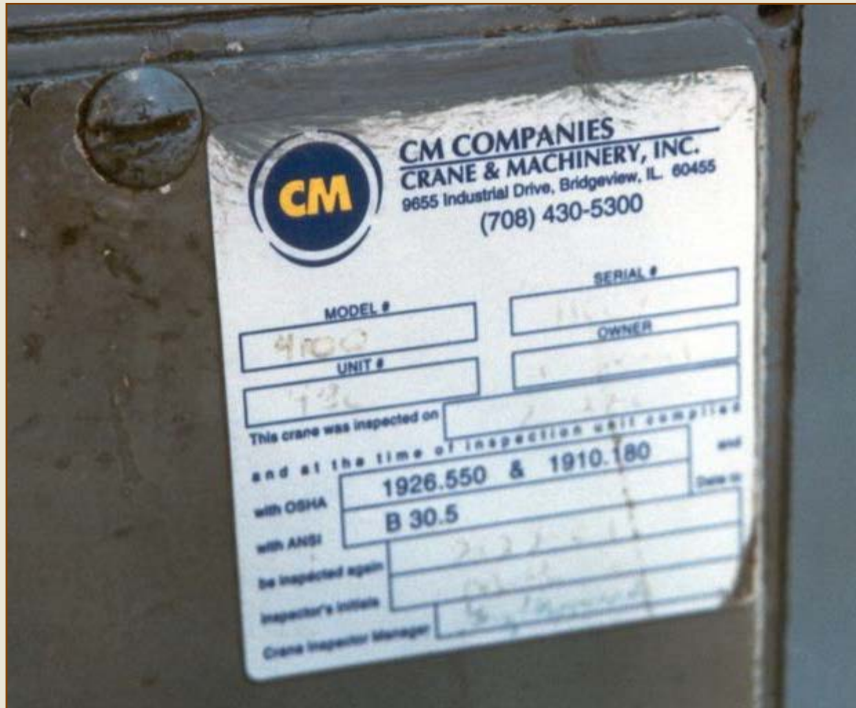
A certification label showing that a crane was recently inspected.
