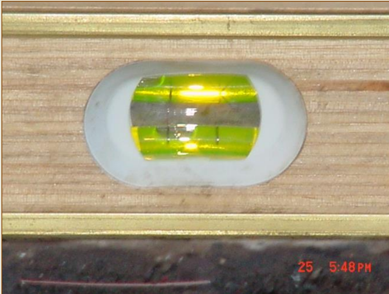
A typical mechanical bubble level in a crane operator's cab. The bubbles are showing that the crane is out of level.
