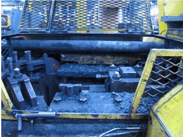
The Interlocked Guard installed after the injury is “Effective Alternative Protection”
