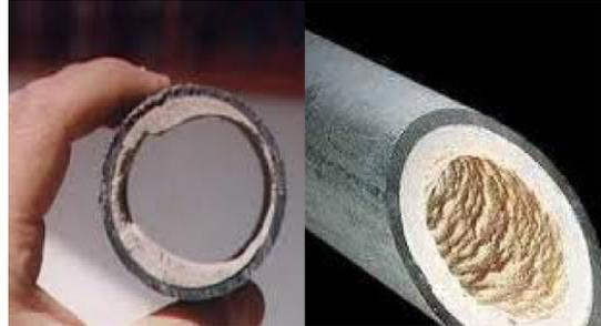
Scale on the inside of a tube
