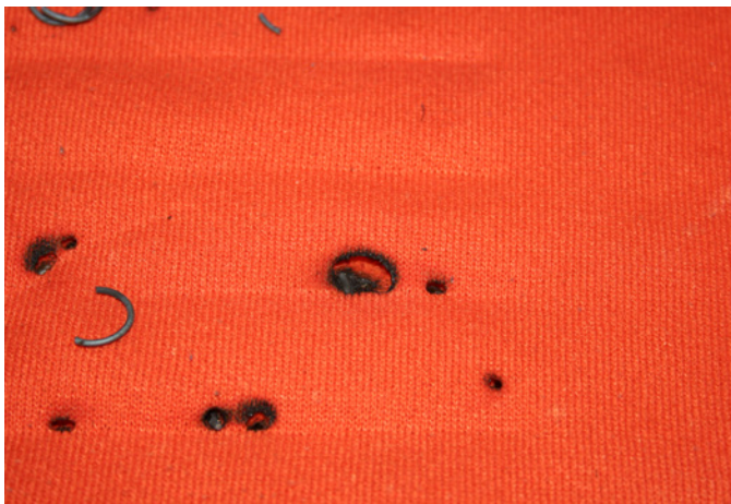
FIGURE 11 Burned spots on sweatshirt under heater with fractured coil
