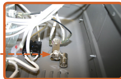
FIGURE 4 Combination thermostat/tip-over switch with polycarbonate plastic arm and arm-pin
