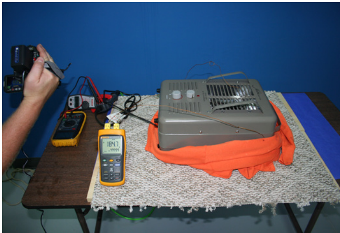
FIGURE 9 Rearward tip over endurance test
