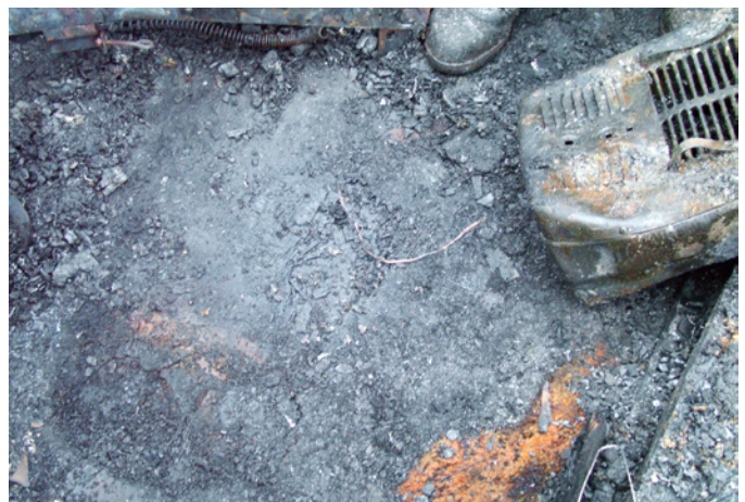
FIGURE 8 Heater No. 1 and floor beneath post-excitation
