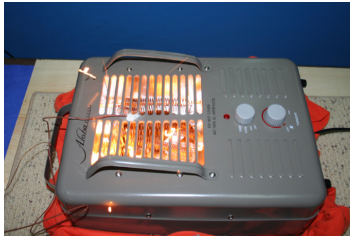
FIGURE 10 Heater at moment of element shorting and fracturing
