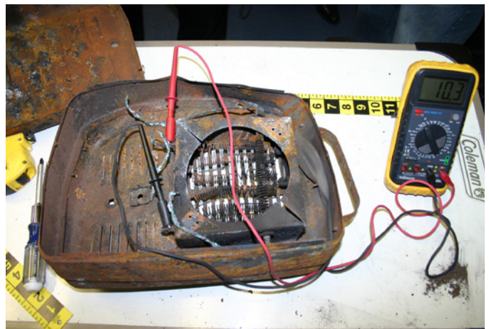
FIGURE 12 Testing of subject heater showed no evidence of shorted heater coils
