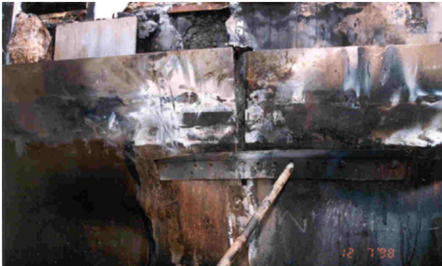
FIGURE 2 Origin area with the wall reconstructed and the left cheese melter hanging bracket held in place.
