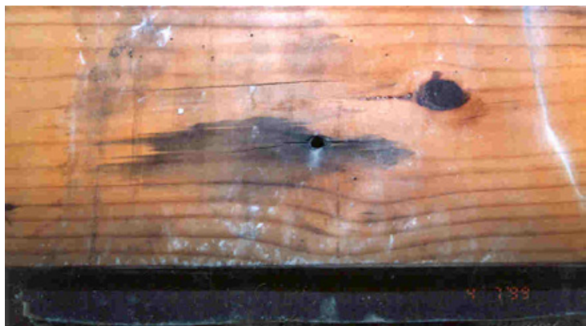
FIGURE 8 Tullahoma, Tennessee. Heat damaged wood blocking where the cheese melter bracket lag bolts penetrated the wall. Wall coverings removed.
