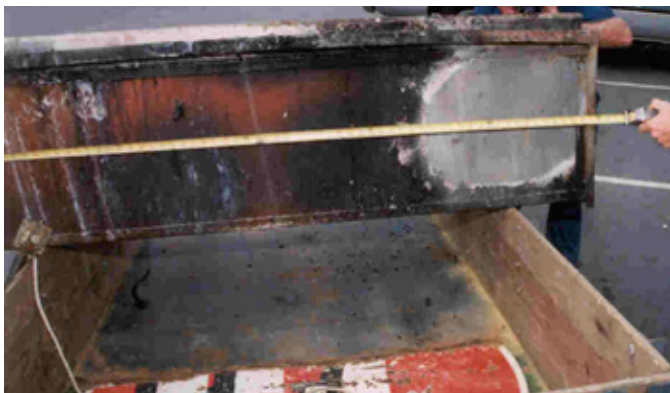
FIGURE 4 A view of the back of the cheese melter. The heat pattern on the right corresponds to the origin area within the wall.
