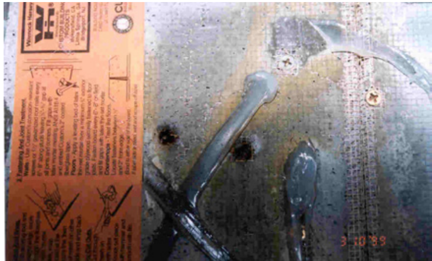
FIGURE 6 Trussville, Alabama. Heat damaged Durock® covering the wood blocking where the cheese melter hanging bracket lag bolt penetrated the wall.
