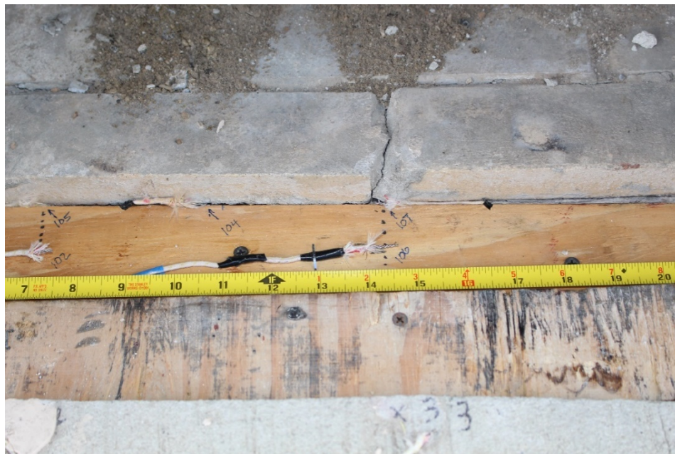
Figure 7: A view of thermocouple locations 104, 105 and 107 located against the top leading edge of the combustibile wood framing undelaying the stucco covering of the hearth extension. Thermocouples 102 and 106 were one inch back from the leading edge. The photograph was taken prior to covering with stucco.
