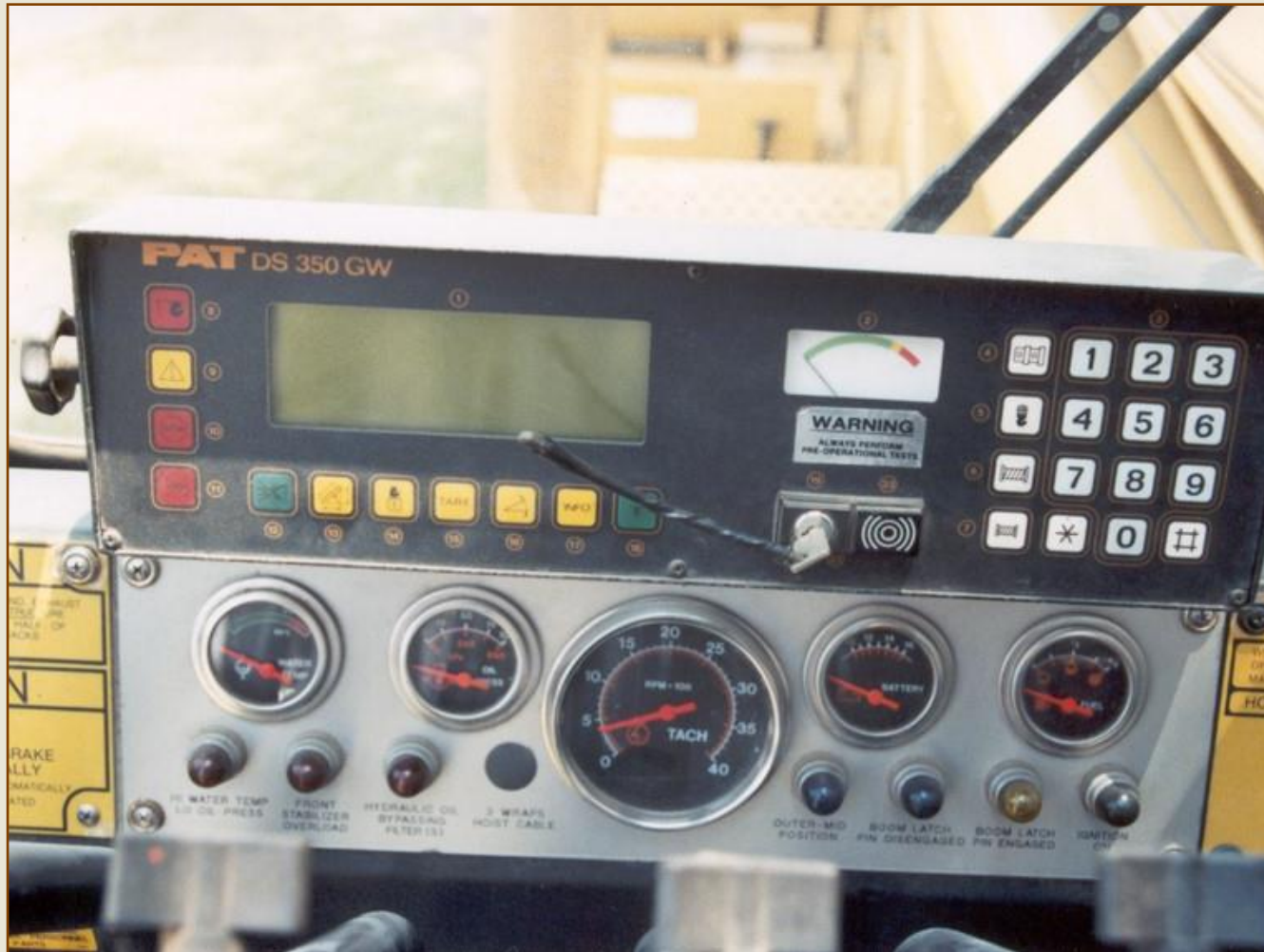
An older Grove PAT LMI (Load Moment Indicator)
