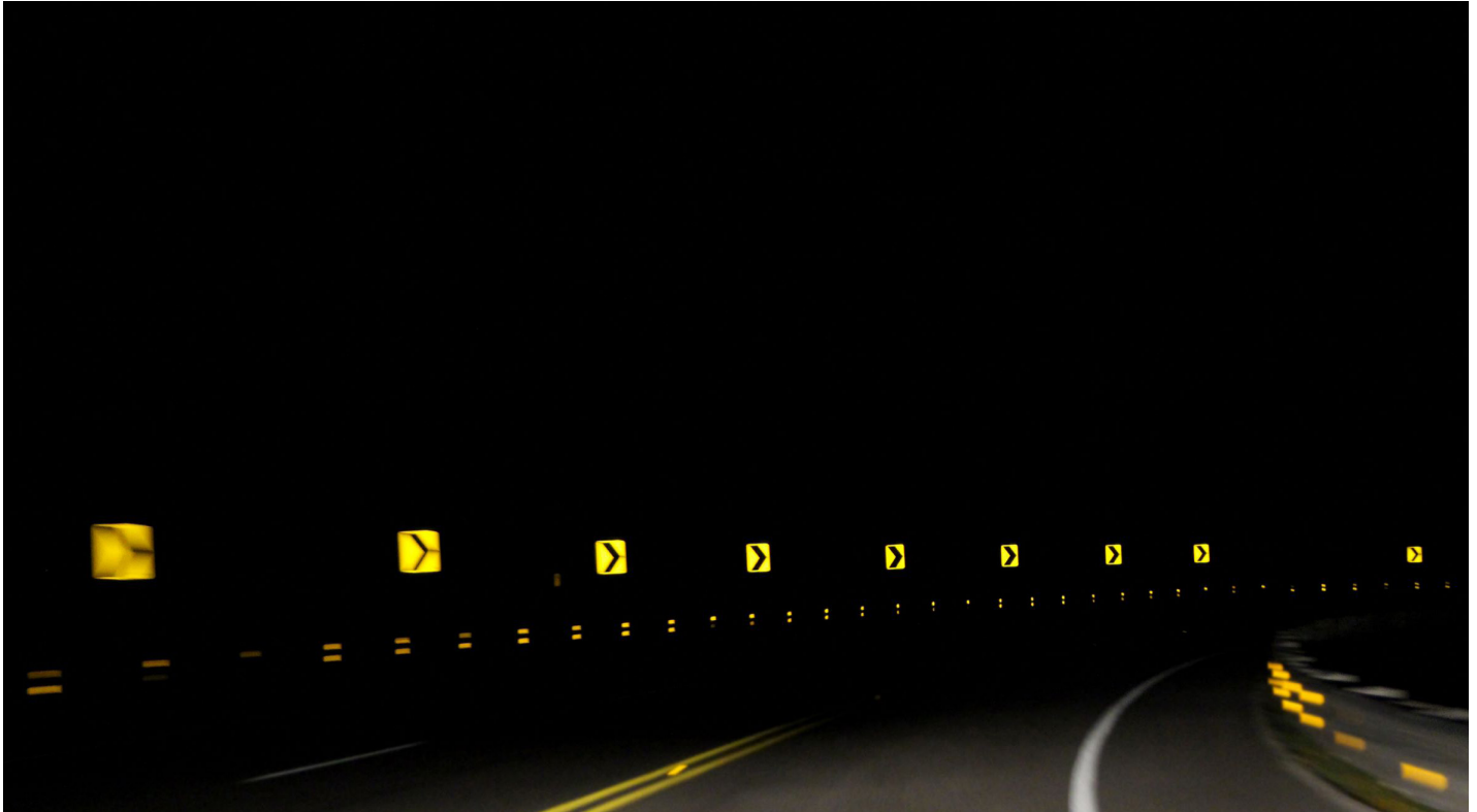
Many road elements, such as lane markings and signs are designed to be highly reflective at night. However, hazards that do not have retroreflective or active lighting properties often lack sufficient contrast to be visible to nighttime
